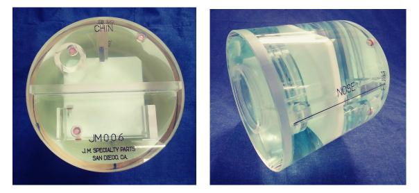
The phantom is an MRI accessory used to evaluate the performance of an MRI machine. HTS: 9018.19.4000
