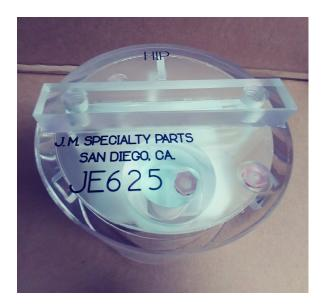
The phantom is an MRI accessory used to evaluate the performance of an MRI machine. HTS: 9018.19.4000
