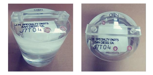
The phantom is an MRI accessory used to evaluate the performance of an MRI machine. HTS: 9018.19.4000
