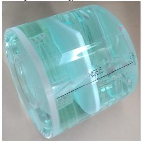
The phantom is an MRI accessory used to evaluate the performance of an MRI machine. HTS: 9018.19.4000
